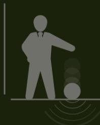
**Impact Insulation Class (IIC)** is a rating of how well a building's floor attenuates impact sounds, such as footsteps.
